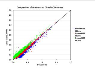
**Figure 5.** Comparison of quasi-simultaneous Brewer and Cimel AOD values from 2006 until 2013.
