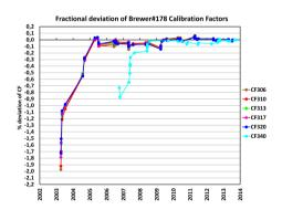
Figure 4. Stability of Brewer#178 Calibration Factors.
